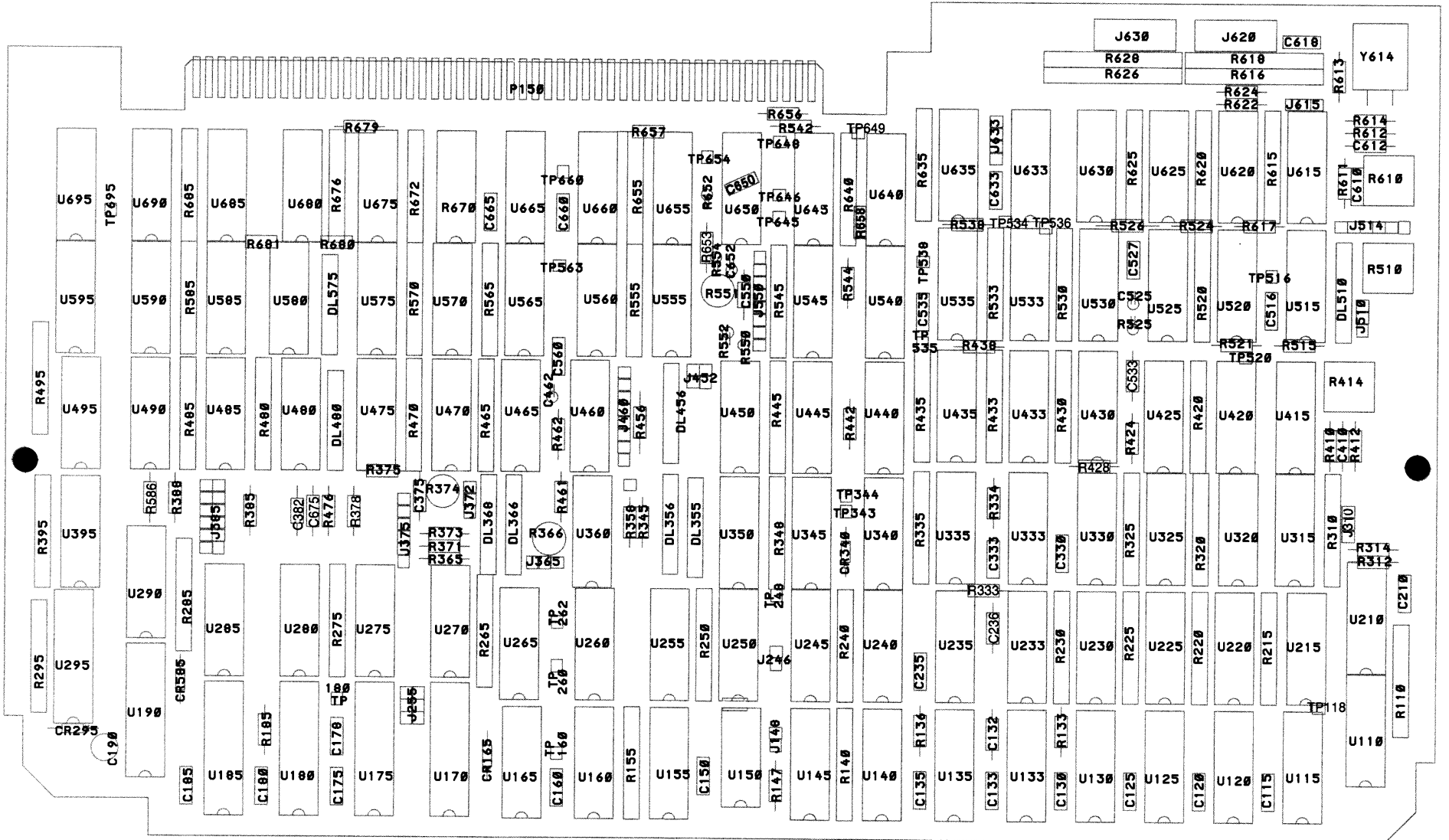
Figure 10-17. A14 Trigger Board Component Locations (870-7523-11).
